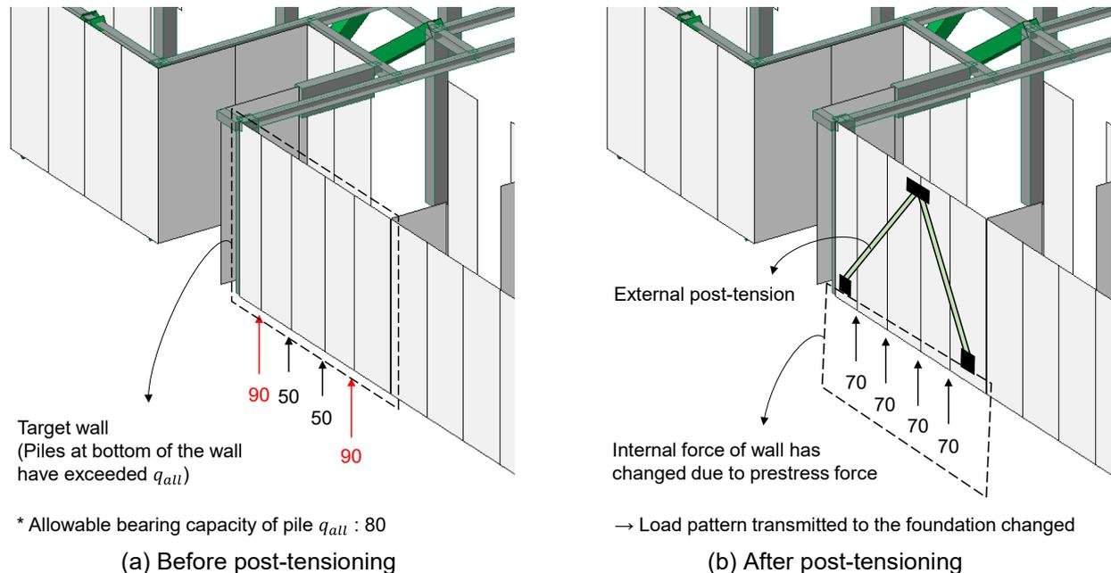
**Fig. 1** Bearing capacity ratio control of piles using external post-tensioning (unit : kN)
