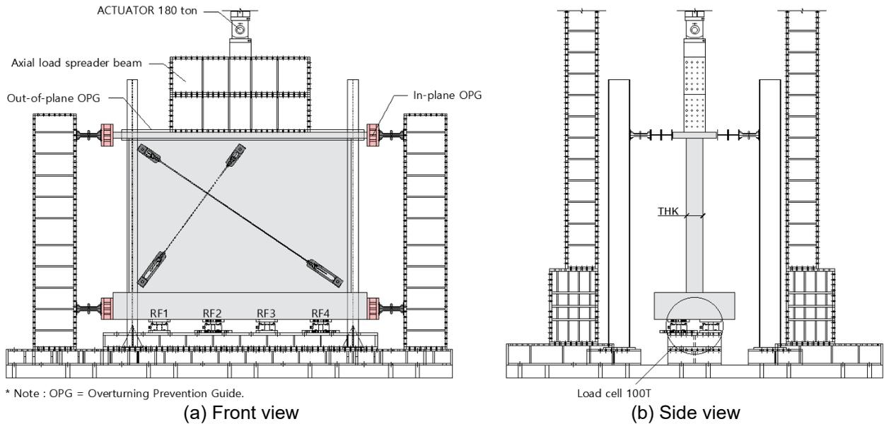
Fig. 2 Test setup
